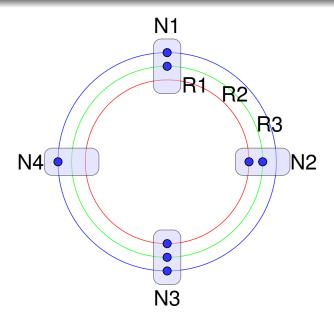
3 rings, 4 nodes, 8 ADMEvery node connected to at least one ringOn every ring are at least two nodes N1 connected to R2 and R3N4 and N2 can't talk to each other Traffic between N1
